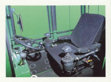
The cabin of the Lokomo 910 has an extremely low noise and vibration level, fully adjustable seat and controls and excellent visibility. These are important for a good working environment, ensuring that the operator can achieve a maximum output with minimum damage and without fatigue.
